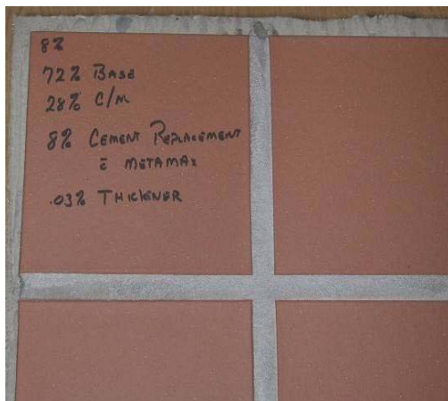
8% MetaMax ® EF @96 hours, Very slight efflorescence
