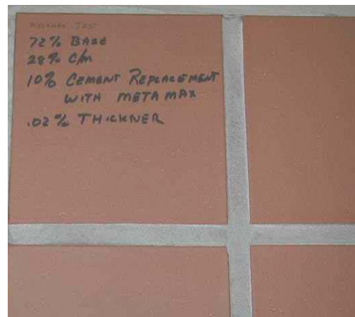
10% MetaMax ® EF @96 hours, None to Very slight efflorescence
